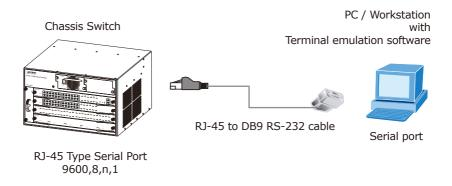
Figure 6-1 XGS3 Chassis Switch Console connection
