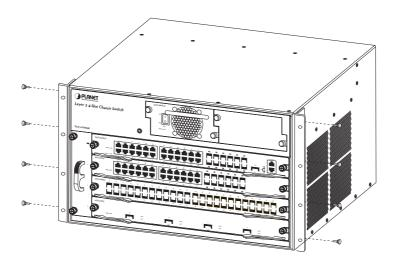
Figure 3-1 Installation XGS3-42000R Rack-mounting Brackets
