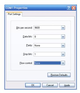
Figure 6-2 Hyper Terminal COM port configuration
