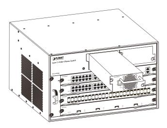
Figure 3-6 Install and Removal the Power Supply Unit
