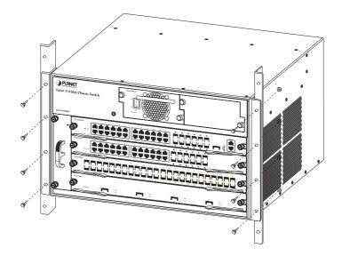
Figure 3-2 Mounting the XGS3-42000R in a Rack
