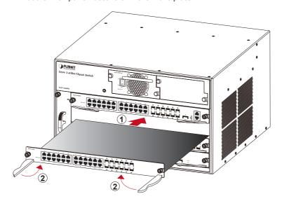
Figure 3-3 Insert the optional module into the slot of XGS3-42000R
