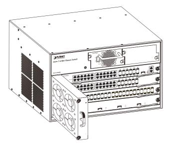
Figure 3-5 Installation and Removal the Fan Tray
